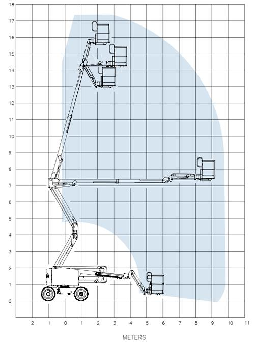
\* The metric equivalent of working height adds 2 m to platform height. U.S. adds 6 ft to platform height.
